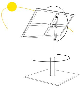
1- or 2-axis tracking systems are used to increase the effectiveness of photovoltaic plants. They align the PV module horizontally and vertically to the sun (azimuth and elevation adjustment). Framo Morat has developed special drive systems for this purpose – in which all components, from the drive housing to the cable, have been specifically designed for harsh outdoor operation.
